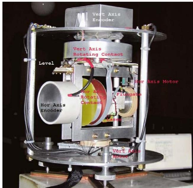
**Figure 1** AUTODIF MKII on the D02 absolute pillar in the Dourbes geomagnetic Observatory. The different elements are indicated
