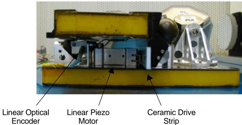
**Figure 9. PAOS Mechanism Rear View**
