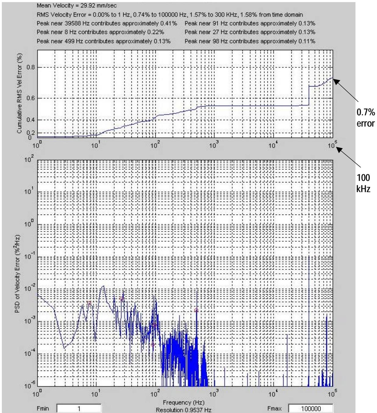
**Figure 16. Velocity Error Data for the PAOS Mechanism**
