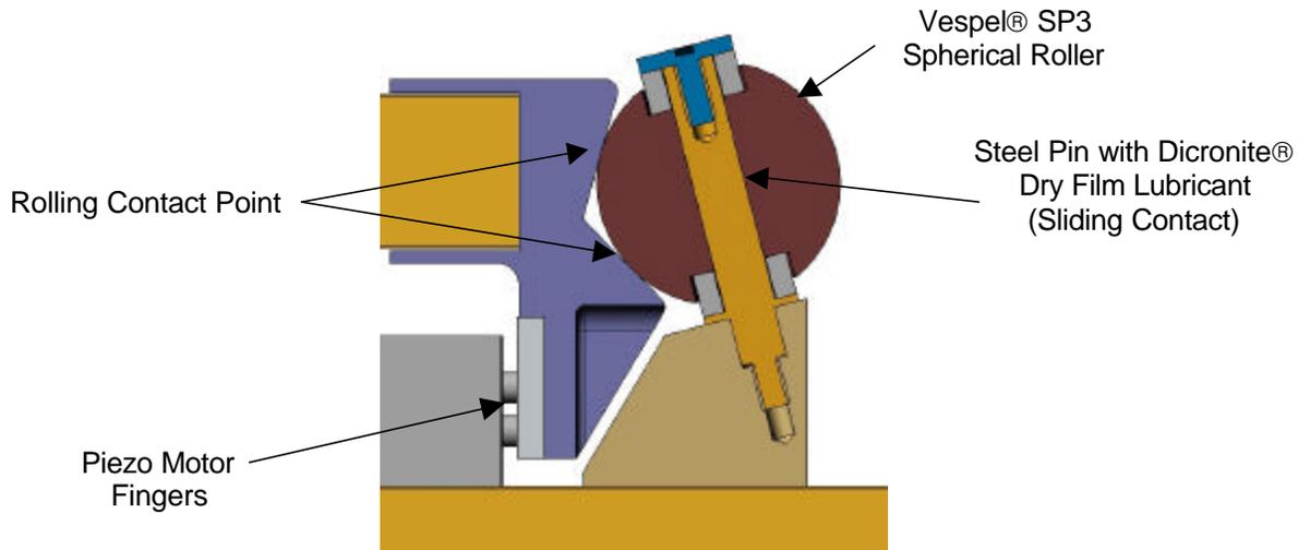
**Figure 12. Spherical Roller Cross Section**
